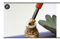
Using a 3/8" T key, remove the tapping tee dust cap and seal
