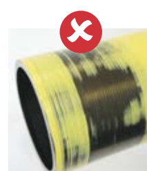
Incorrect pipe preparation for electrofusion
