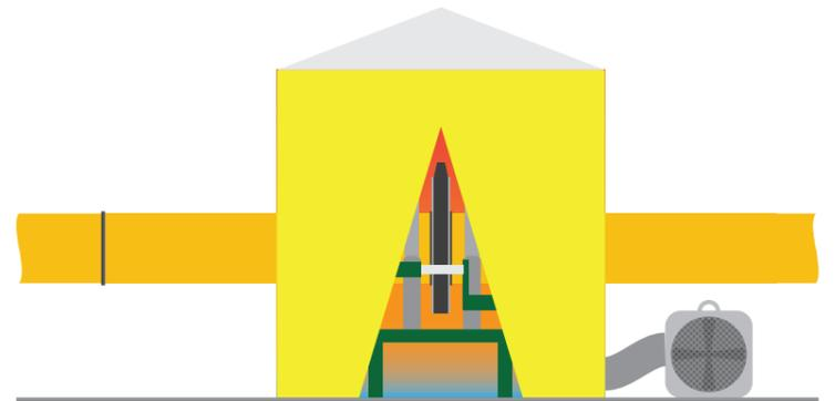
The butt-fusion equipment is pre-programmed with welding parameters depending on the pipe's material, diameter and SDR, based on ambient temperatures of  $0^{\circ}\text{C}$  and above, as identified in the UK water specification, or  $-5^{\circ}\text{C}$  and above as required by the UK gas industry.
