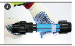
Push the pipe fully into the body of the fitting
