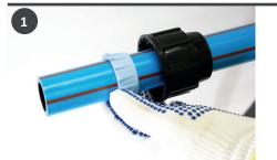
Ensure the pipe is cut square and damage free. Re-round if necessary. Slide the nut and grip ring on the pipe
