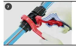
Using C ring wrenches fully tighten the nuts onto the body of the fitting
