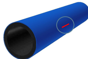
Fig 4. Critical areas of squeeze off Critical areas are located 90° to the squeeze tool compression bars, extending 100 mm either side of the bars and a distance 'Y' around the circumference of the pipe (see Fig.5). 'Critical areas' should be free from pipe damage or pipe surface damage.
